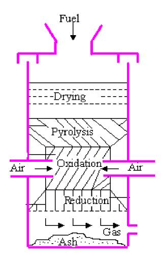
Fig.2 Downdraft Gasifier
